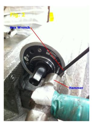
2. Use Hammer and Hex Wrench to knock the both heads of Bolt B to release BB2008-1.(See Fig.2)
