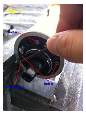
1. Release both Bolt B and bolt A with Hex Wrench for 2-3mm. (See Fig.1)
