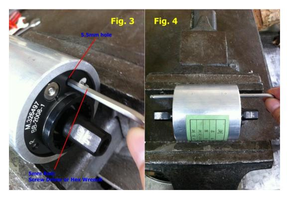
3. Insert 5mm Rod through into 5.5mm holes from left to right.(See Fig.3 $^{\sim}$ 4)
